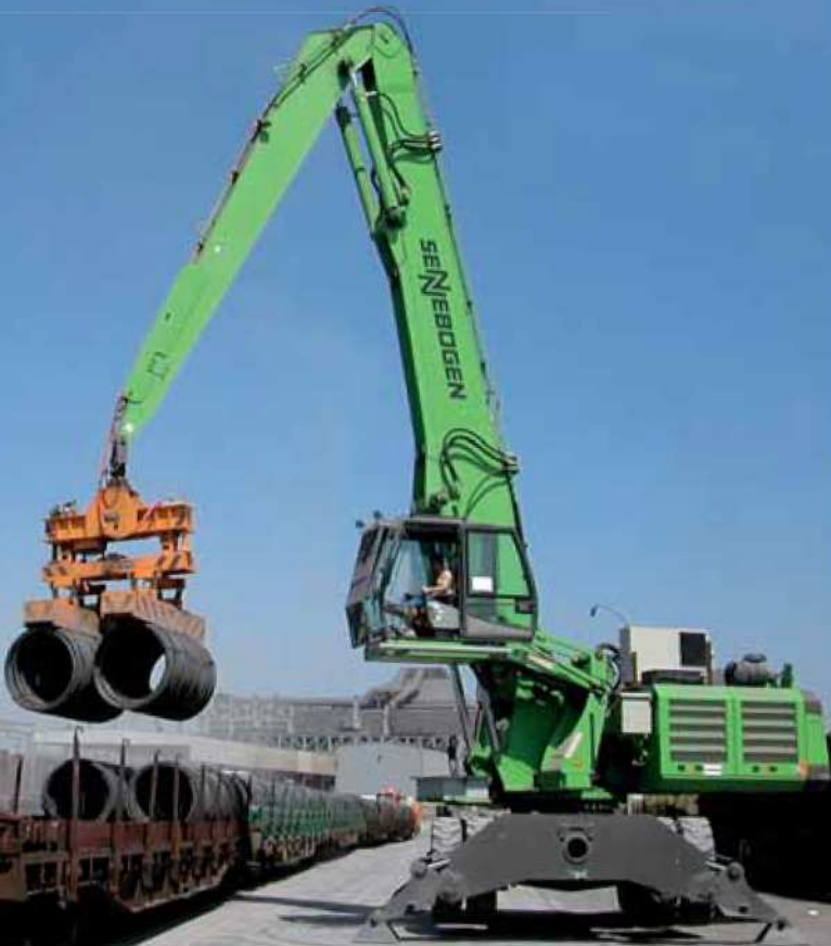
870 M - Ausrüstung K20 - Magnettraverse - Spanien 870 M - equipment K20 - magnet device - Spain
