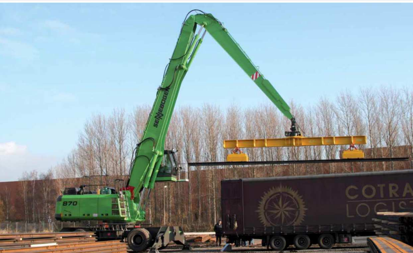
870 M - Ausrüstung K18 - Magnettraverse - Russland 870 M - equipment K18 - magnet device - Russia
