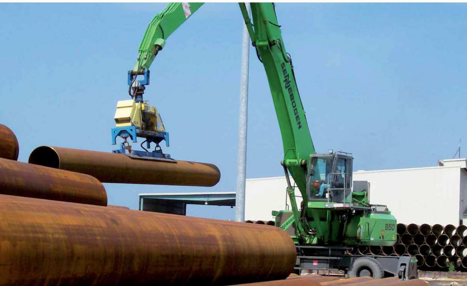
850 M - Ausrüstung K17 - Vakuumtraverse - USA 850 M - equipment K17 - vacuum lifting device - USA
