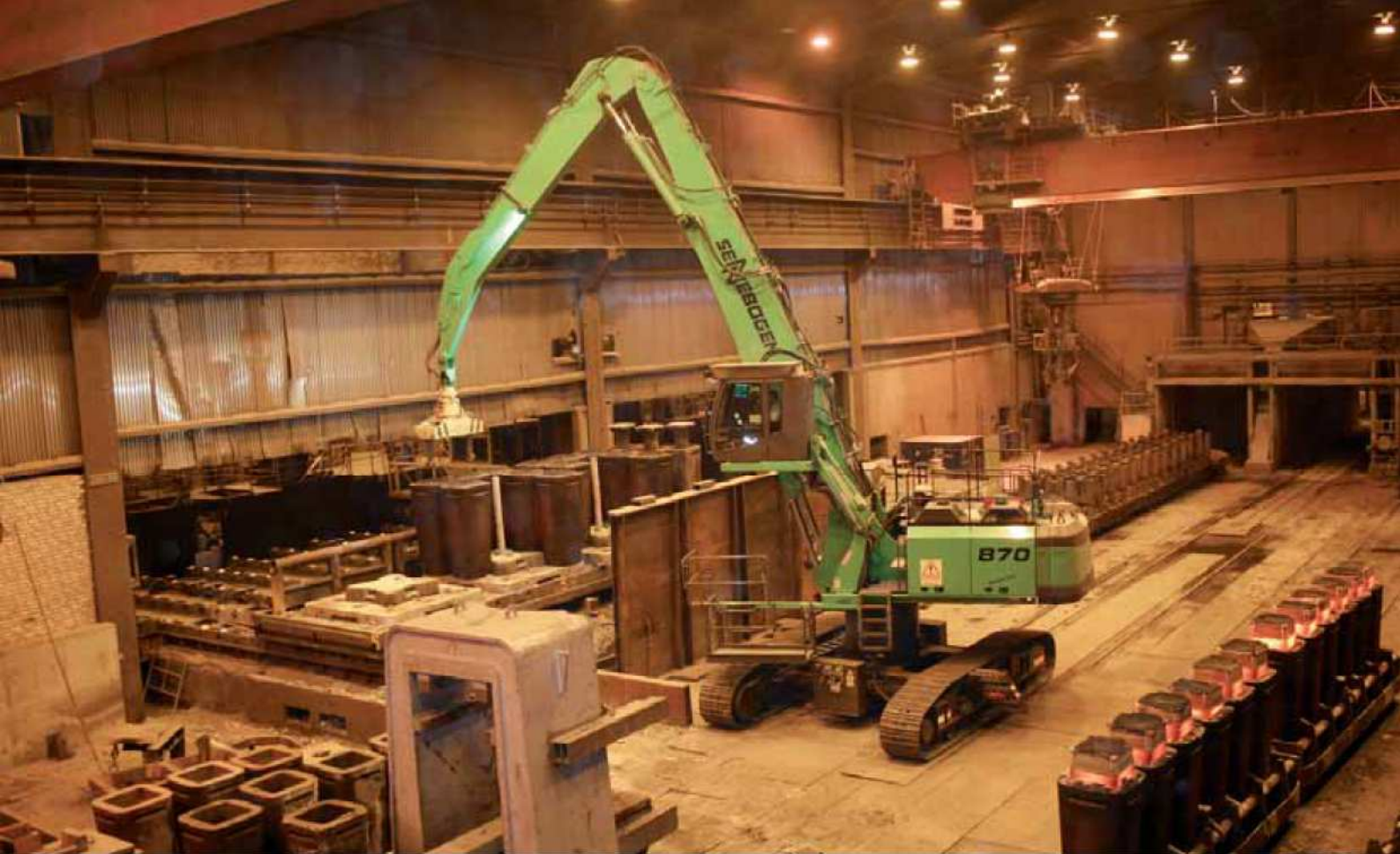
870 R spezial – Elektro – 1 m Pylon – Sonderausrüstung K17 – Kokillentraverse – Schweden 870 R special – electro – 1 m pylon – special equipment K17 – ingot mould lifting device – Sweden
