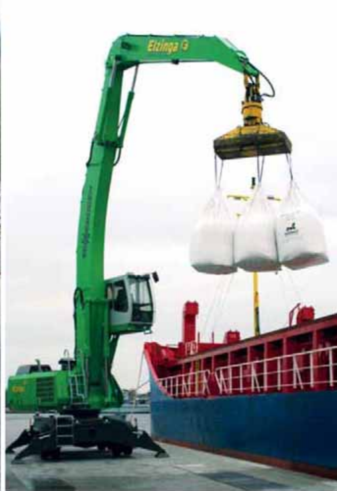
835 Mobile - B18 equipment, big bag handling; Netherlands 835 Mobil - Ausrüstung B18, Big Bag-Verladung; Niederlande
