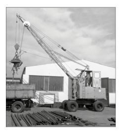
1962: rope-driven S833 with elevated operator cab
