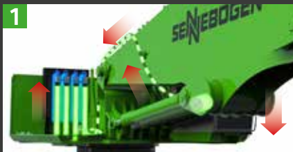
1 Boom lowers, gas compresses
