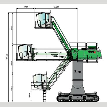
850 R special with R70/490 undercarriage and 3.0 m pylon, Mastercab Skylift 900 can be elevated hydraulically R
