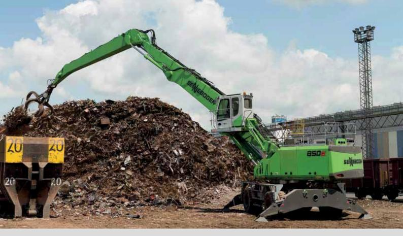
850 M - with orange peel grab - scrap handling; Austria
