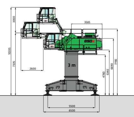
850 special with 4-point ST78/550 pedestal and 3.0 m pylon, Maxcab E300/260 can be elevated and moved forward hydraulically
