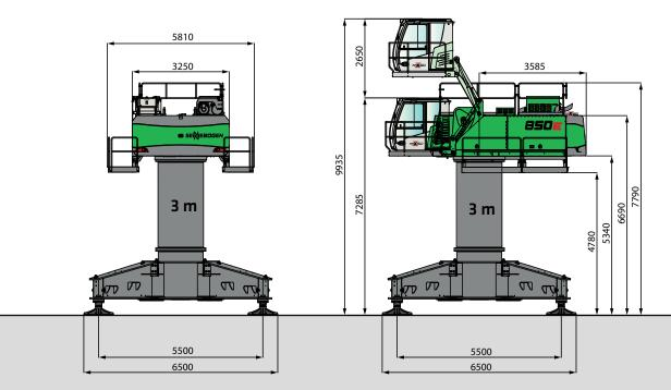
850 special with 4-point ST78/550 pedestal and 3.0 m pylon, Maxcab E270 can be elevated hydraulically R
