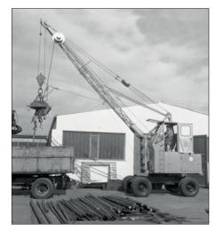
1962: Rope-driven S833 with elevated operator cab
