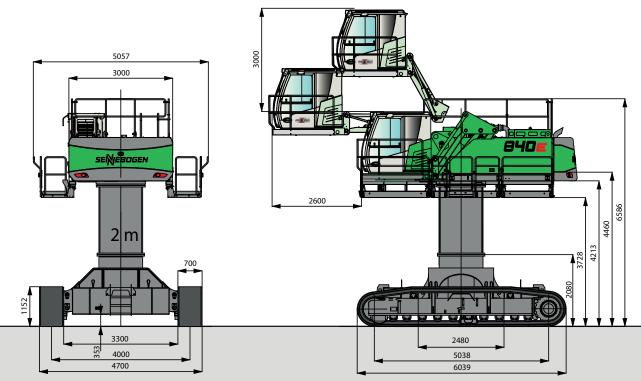
840 R with wide-gauge undercarriage type R44/400 and cab elevation E300/260, Maxcab can be elevated and moved forward hydraulically
