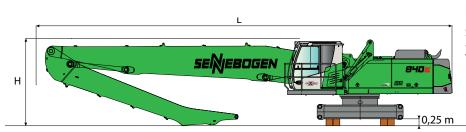
Crawler tracks (type B7) for undercarriage R44/380 with 700 mm grouser track shoes, Weight: approx. 7600 kg each, 2 pieces
