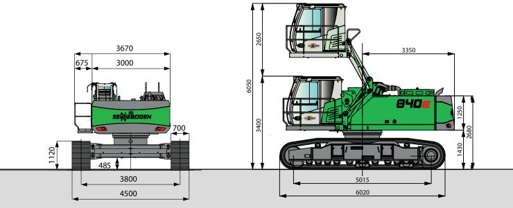
840 R with wide-gauge undercarriage R44/380 and cab elevation E270, Maxcab can be elevated hydraulically
