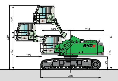
840 R with wide-gauge undercarriage R44/380, cab elevation type E300/260, Maxcab can be elevated and moved forward hydraulically
