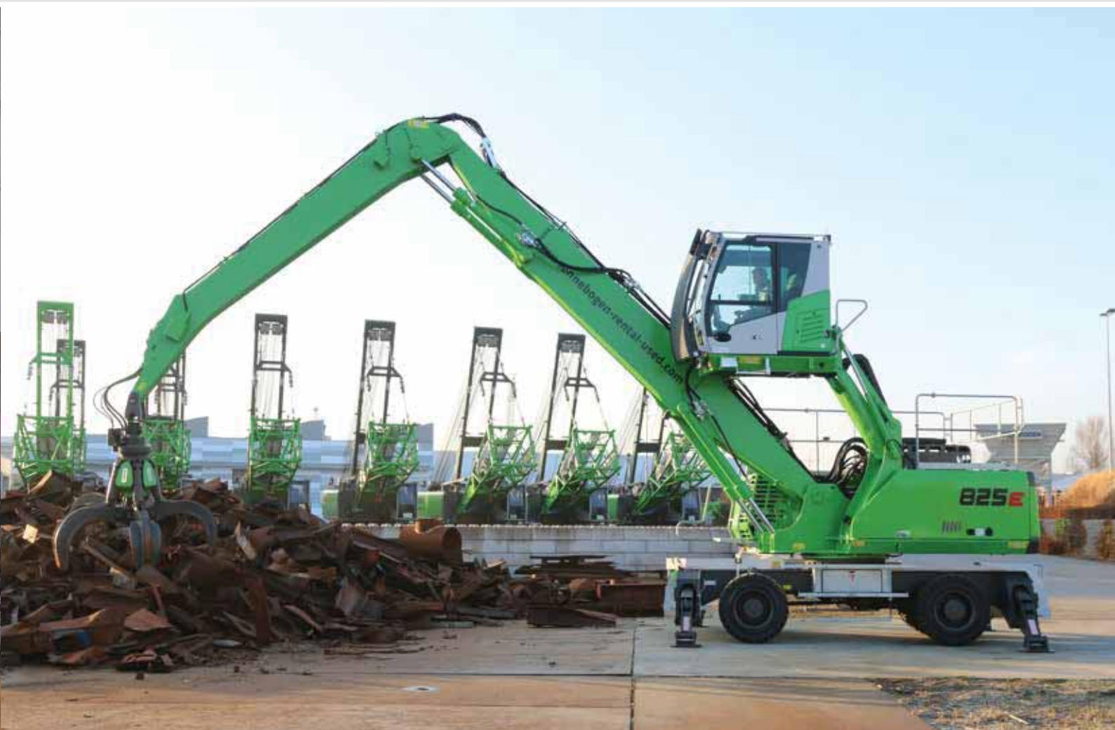
825 M - Mobile scrap handling with original SENNEBOGEN orange peel grab; Germany
