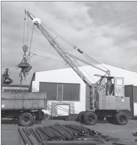
1962: rope-driven S833 with elevated operator cab
