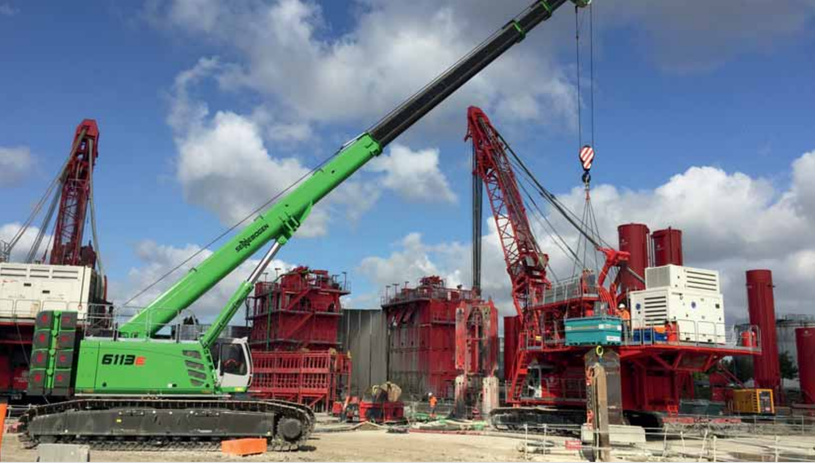
6113 R - high stability on any site surface with Star-Lifter broad gauge chassis; Germany
